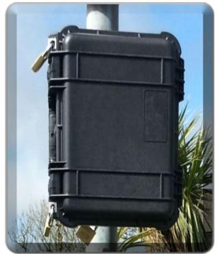
2.1.2 The principal role of the unit is to detect, and count passing vehicles and log the date, time and speed at which they passed. Data collected can be used to determine the volume of traffic flow on the road on which the unit has been deployed.
